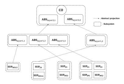
Fig. 4. Control architecture resulted from our approach
