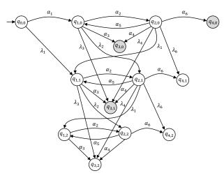
Fig. 2: Security automaton of the plant in Figure 1 with  $\ell(q_0) = \ell(q_1) = \ell(q_2) = 0$ ,  $\ell(q_3) = 2$ ,  $\ell(q_4) = 1$ .
