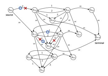
Fig. 5: The s-t graph  $\mathcal{G}$  of the SA in Figure 2 with costs 2, 1, 1, 3, 1,  $\infty$ , respectively for events  $\sigma_1, \sigma_2, \sigma_3, \sigma_4, \sigma_5, \sigma_6$ . The "blue circles" denote the arcs in the s-t min-cut  $\mathcal{C}_{min}$  in Example 5.2, which are different from the "red crosses" denoting the disablement of events by supervisor  $\xi_{max}$  in Example 4.2.
