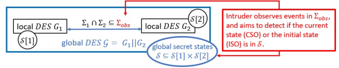
Fig. 1. An overview of our distributed architecture with two local DESs. The global DES \mathcal{G} is the parallel composition of local DESs. The secret state set \mathcal{S} is a set of states of \mathcal{G} . We assume that the events shared by the local DESs are observable by the intruder ( \Sigma_1 \cup \Sigma_2 \subseteq \Sigma_{obs} ). The objective of the intruder is to detect if the current state (for the CSO problem) or the initial state (for the ISO problem) of \mathcal{G} is in \mathcal{S} (see Section III). Note that this architecture can be extended to n local DESs.
