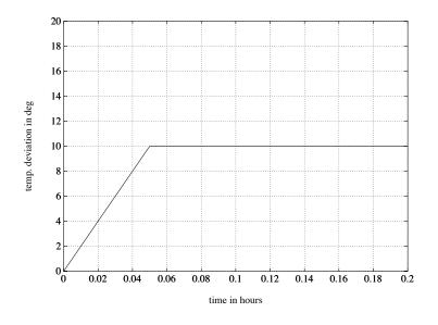
This disturbance is acting on the measured variables,  $T_{14}, T_{28}$ ; this is referred to as "equivalent output disturbance".
