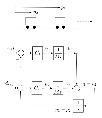
Car 1 has the model  $M\dot{v}_1 = u_1$ ; likewise for car 2. Controller  $C_1$  has input the speed error, while controller  $C_2$  has input the relative position error. The symbols  $v_i$  stand for speed and  $p_i$  for position.
