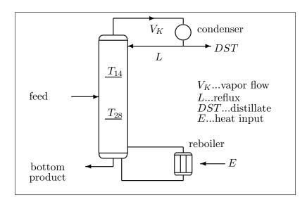
Figure 1: Schematic representation of distillation column
